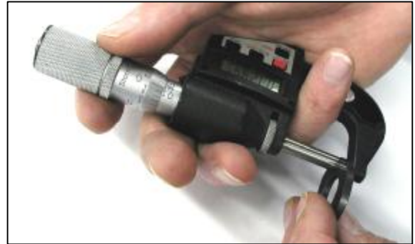
Measuring Wear Plate Thickness
