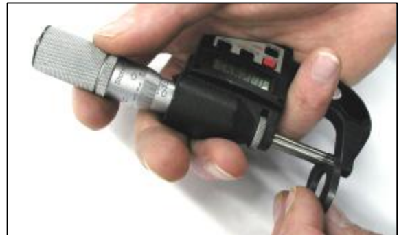
Measuring Wear Plate Thickness
