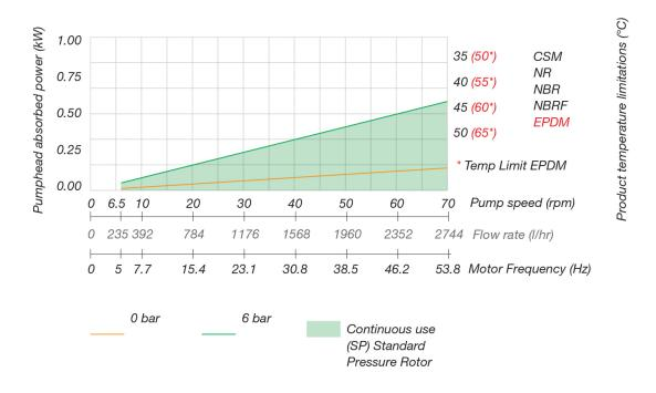
Actual flows will vary according to suction conditions, discharge pressure and normal component production tolerances.
